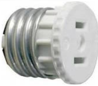
Figure 9: Screw-in receptacle recommended to replace FUSE B for 115 volt operation. The receptacle may be used as a switched AC outlet.
