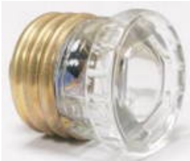
Figure 5: Old style screw-in fuse as used in the KS-1. Two 15 A fuses are required for 230 volt operation and one 25 A fuse is required for 115 volt operation.
